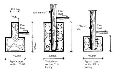
Figure 15: Details of the footings Illustraion by Duval Zambrano/J. Cuizano
